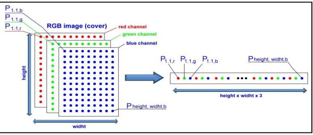
Fig. 8. Converting a color image to a one-dimensional array
