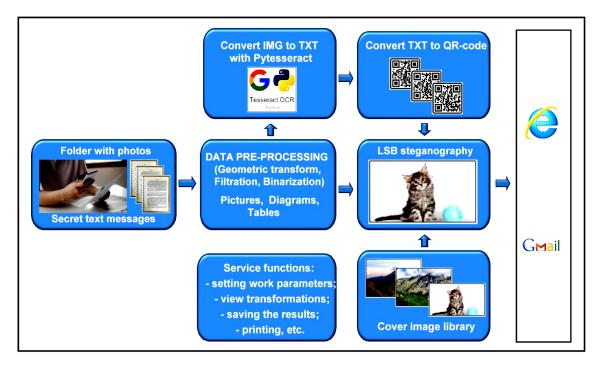
Fig. 3. Structure of the optical text recognition system with protecting information identified
