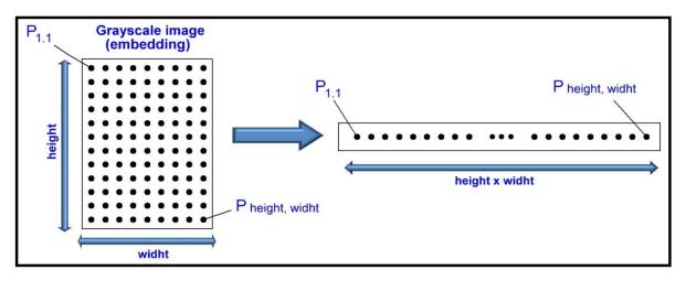
Fig. 7. Converting a grayscale image to a one-dimensional array
