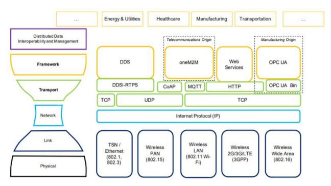
Fig. 1. Interconnection standards in IIoT [12]
