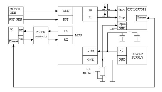
Fig. 1. A functional diagram of the source system modeling of information from microprocessor from digital device
