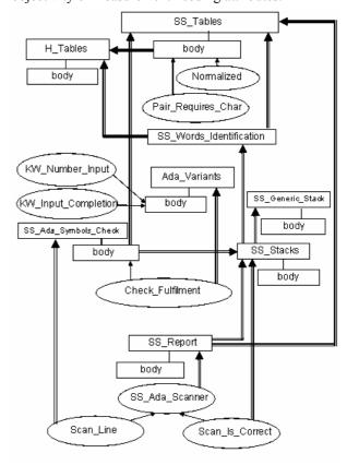
Fig. 1. The scheme of program structure (SPS) for  $SS\_Ada\_Scanner$  that help us count tokens of programs
