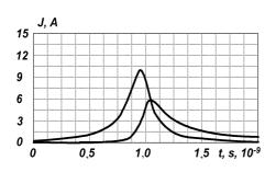
Fig. 5. Dependencies of the discharge current (upper curve) and plasma electron current (lower curve)
