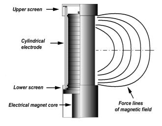
Fig. 2. Scheme of the cylindrical probe
